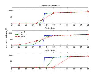
Output for different discretization schemes and step-sizes
